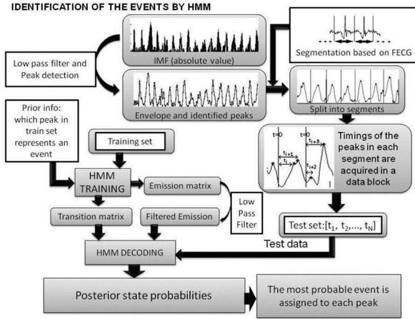
Fig. 3. HMM approach block diagram.
