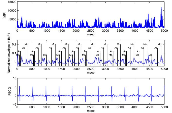
Fig. 8. Example of identified events: mitral opening and closing (Mo and Mc) and aortic valve opening and closing (Ao and Ac).
