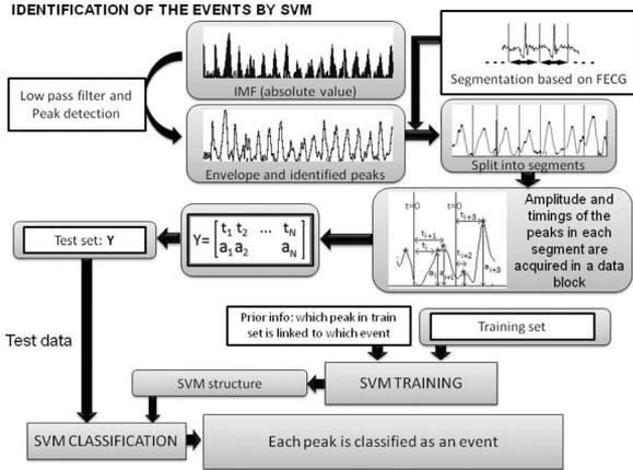
Fig. 4. SVM approach block diagram.
