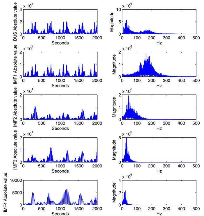
Fig. 2. Decomposition of the DUS signal using EMD.
