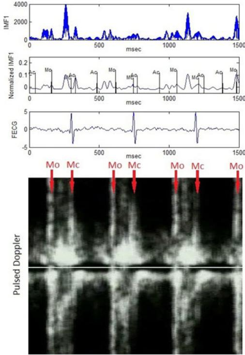
Fig. 6. (a) First IMF of the DUS signal decomposed by EMD. (b) Envelope of the normalized IMF and the identified timings. (c) The simultaneous fECG signal extracted from abdominal ECG signals using BSSR. (d) Pulsed wave Doppler signal of fetal mitral valve movements annotated to show how the specific signals are linked with opening and closing events. Mo and Mc represent the opening and closing of mitral valve.
