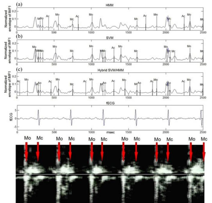
Fig. 9. Comparison of the identification of the valve movements by using (a) HMM, (b) SVM and (c) Hybrid SVM/HMM.
