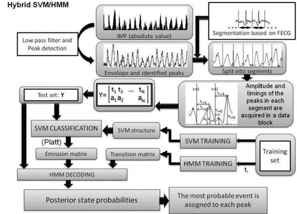
Fig. 5. Hybrid SVM-HMM approach block diagram.
